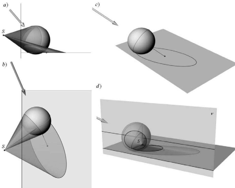
Figure 2: The same example of the shadow of the sphere in linear perspective in 3D modeling software Rhinoceros – a) front view, b) top view, c) situation in the space, d) situation in the space with the determination of linear perspective ( $S$  is the center of the projection and  $v$  is the projection plane) and the projected image. In a), b), d) there are also illustrated imaginary cones of perspective sight. In every picture the arrows define the directional light.
