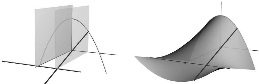
Figure 7: Illustration of the generation of ruled surfaces by a moving straight line. This is the special type of ruled surface which is called a parabolic conoid. Straight lines on the surface are parallel with the depicted plane and intersect parabola and straight line. On the left input elements, on the right the final shape of the conoid.
