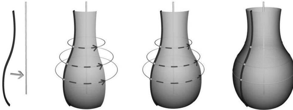
Figure 5: Illustration of the generation of surface of revolution by rotating a curve about an axis. Every point of the curve describes a circle with the center on the axis.
