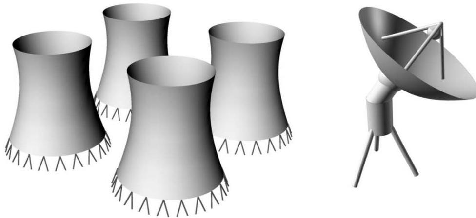
**Figure 8:** Examples of practical uses of surfaces of revolution; on the left the one-sheet rotational hyperboloids as cooling towers, on the right the rotational paraboloid as radio telescope.
