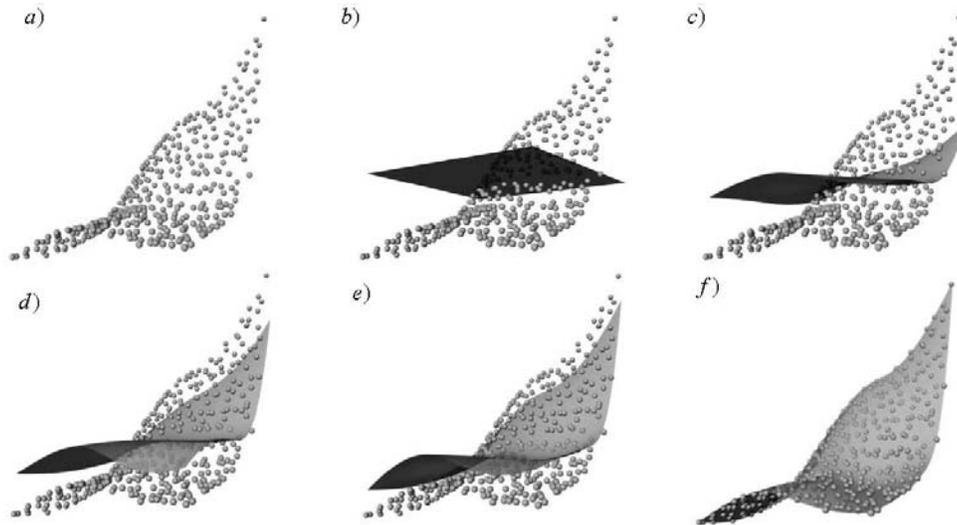
Figure 13: The illustration of sequential evolution – a) the input point cloud in the space, b) initial position and shape of the surface and the input set of points, c) – e) surface evolution in time, f) the final surface
