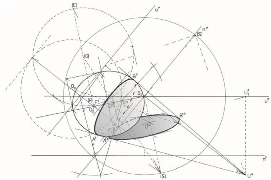
Figure 1: The shadow of the sphere in linear perspective. The situation in two dimension obtained by projection of the sphere into the plane, the picture is hand-made.
