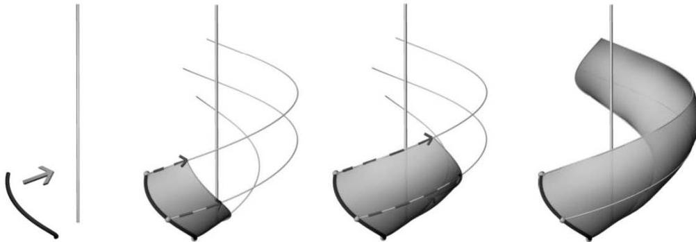
Figure 6: Illustration of the generation of helical surfaces by helical motion a curve about an axis. Every point of the curve describes a helix with the same axis as the axis of surface.
