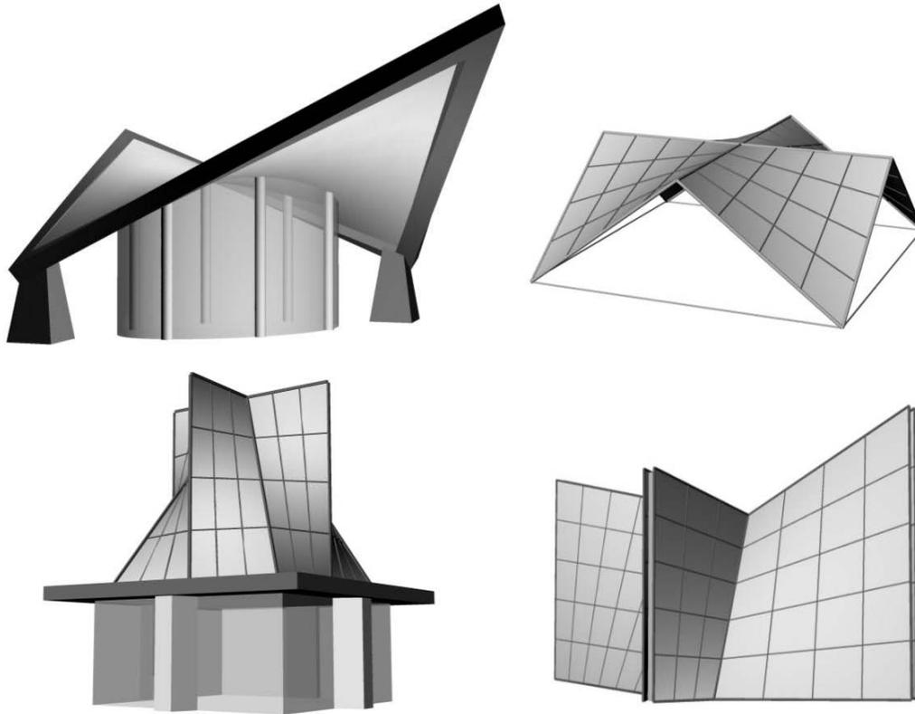
Figure 10: The hyperbolic paraboloids in use by architectural design.
