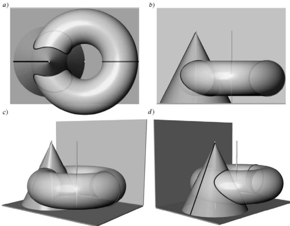
**Figure 4:** Intersection curves of two surfaces of revolution – a) top view, b) front view, c) and d) two perspective projections of intersection curves of two surfaces of revolution.
